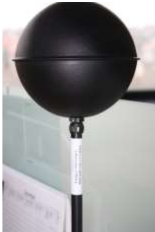
TESTO 6055/0600 9999 radiation temperature measurement equipment
